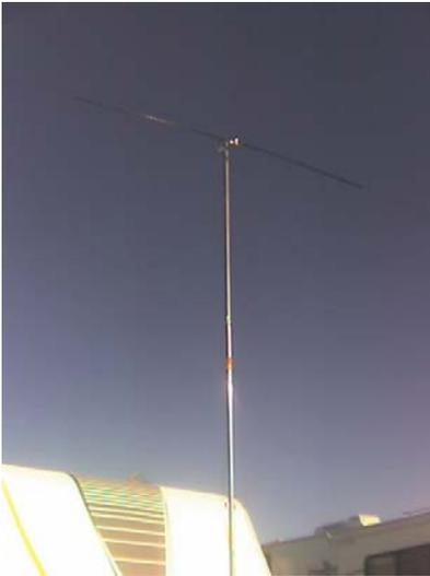
was less than four feet. Fully extended, the 18 foot vertical mounted in the center of the roof was an excellent antenna. The trailer had a ladder on the back that made getting onto the roof for mounting, easy and quick. With practice I got to the point where I could install the vertical on the roof of the trailer in less than 5 minutes. Very nice for making the evening CW contacts and listening on the bands.
