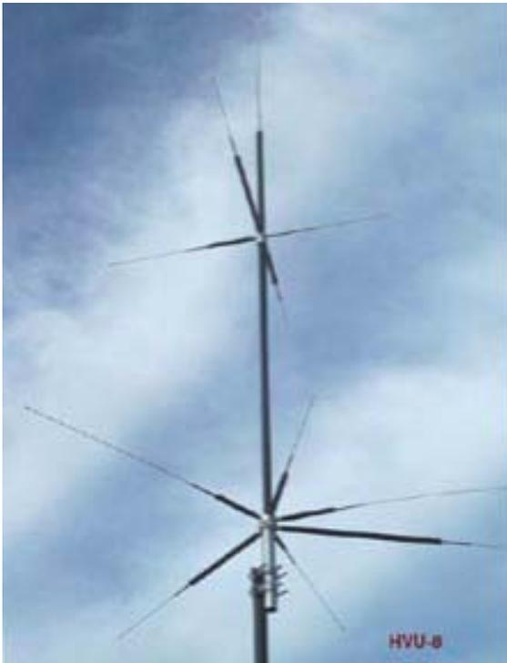
The antenna was made to cover the following bands – 80/40/20/15/10/6/2m and 70cm bands. While experimenting with the antenna (like all good Hams do) I found out that I was able to tune the 60/30 meters band with no problem by using a tuner.
