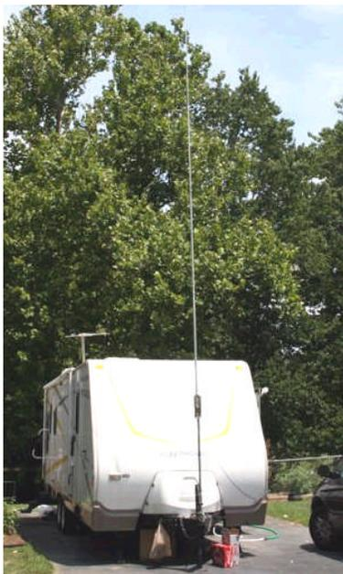
Here are two photographs of the generator installation and vertical antenna on the trailer before leaving Easton, Maryland. I cleverly hid the generator under a weber grill cover - not wanting to tempt someone. The vertical antenna provides 80-6 meter operation with no tuning. It has proved to be an adequate antenna - and so very simple to setup
